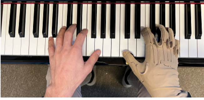
Fig. 1: Experimental setup of one subject playing the piano while kinematic data of their right hand was recorded with a CyberGlove.
